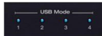
**IMPORTANT:** Please allow at least 1 minute for new USB signal flow to establish after moving the USB mode switch. During this transition, HDBaseT input and output connections may temporarily drop.
