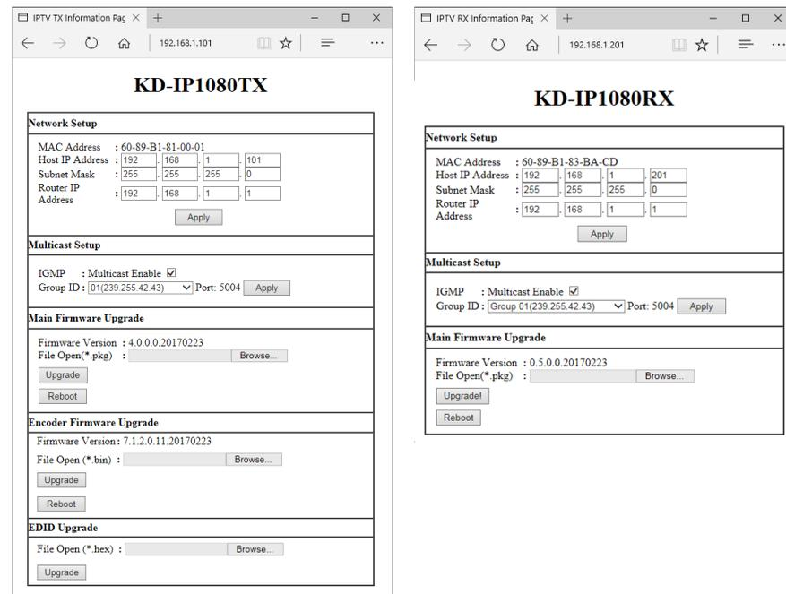
Once connected, the KD-IP1080 web interface would look like this (**Tx on left, Rx on Right**). Network Setup, Multicast Setup, and Main Firmware Upgrade are the same for both Tx and Rx units.
