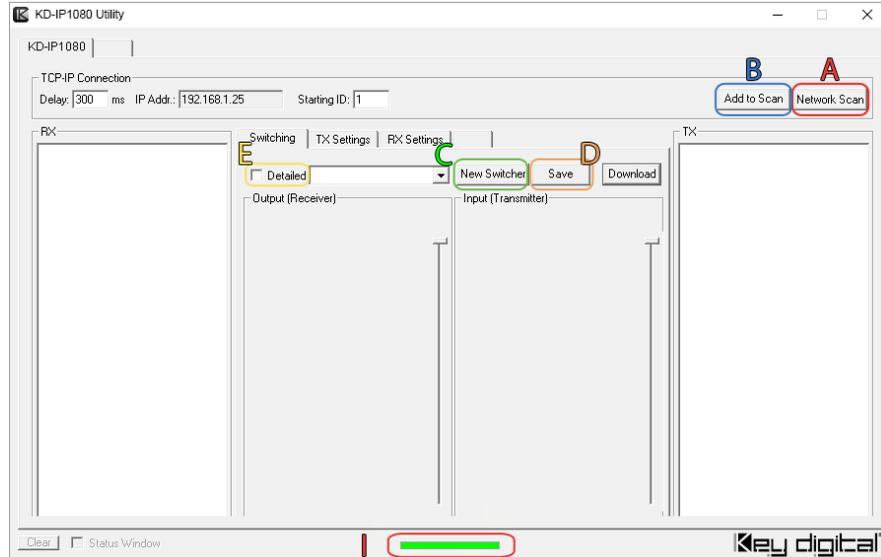
After scanning is complete (**the status bar must be green, Indicator I**), select “New” (**Indicator C**) and a pop-up window will appear. Insert a name for the system (**Indicator F**), example: `switcher_8x24`, and insert the number of inputs/outputs in its respective text field then click “OK”.
