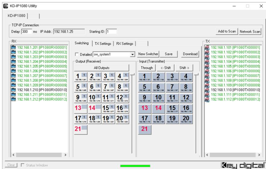
Once all units are discovered and configured, click “Detailed” to be checked off to have basic control of the matrix system (**Indicator E**). To switch sources, select a Output first then select an Input.
