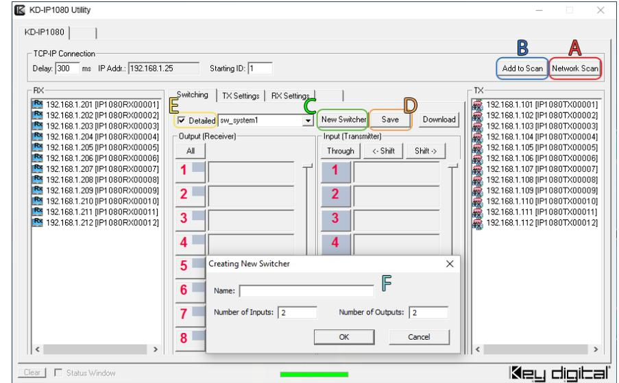
Once the file is created, all inputs/outputs will auto populate. Drag and drop Rx units into an Output Number and Tx units into an Input Number.
