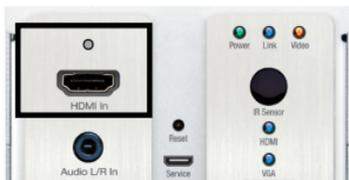
**HDMI Input:** Using an HDMI cable, connect your HDMI source. For DVI-D/DVI-I sources, use appropriate adapters. For Display Port, use active adapters
