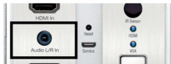
**Analog L/R Input:** Using a 3.5mm stereo cable, connect your audio source to be associated with the VGA video input.
