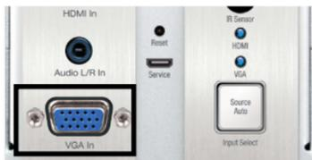
**VGA Input:** Using a Male 15pin VGA cable, connect your VGA source.
