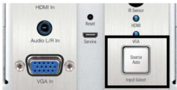
**Input Select Button:** Used to toggle between VGA or HDMI source input or to activate Auto Switch mode.
