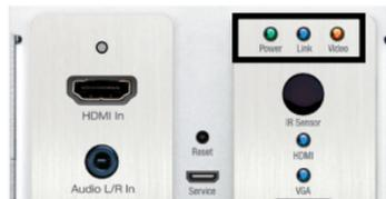
**Power, Link, Video LEDs:** Indicate system connectivity status
